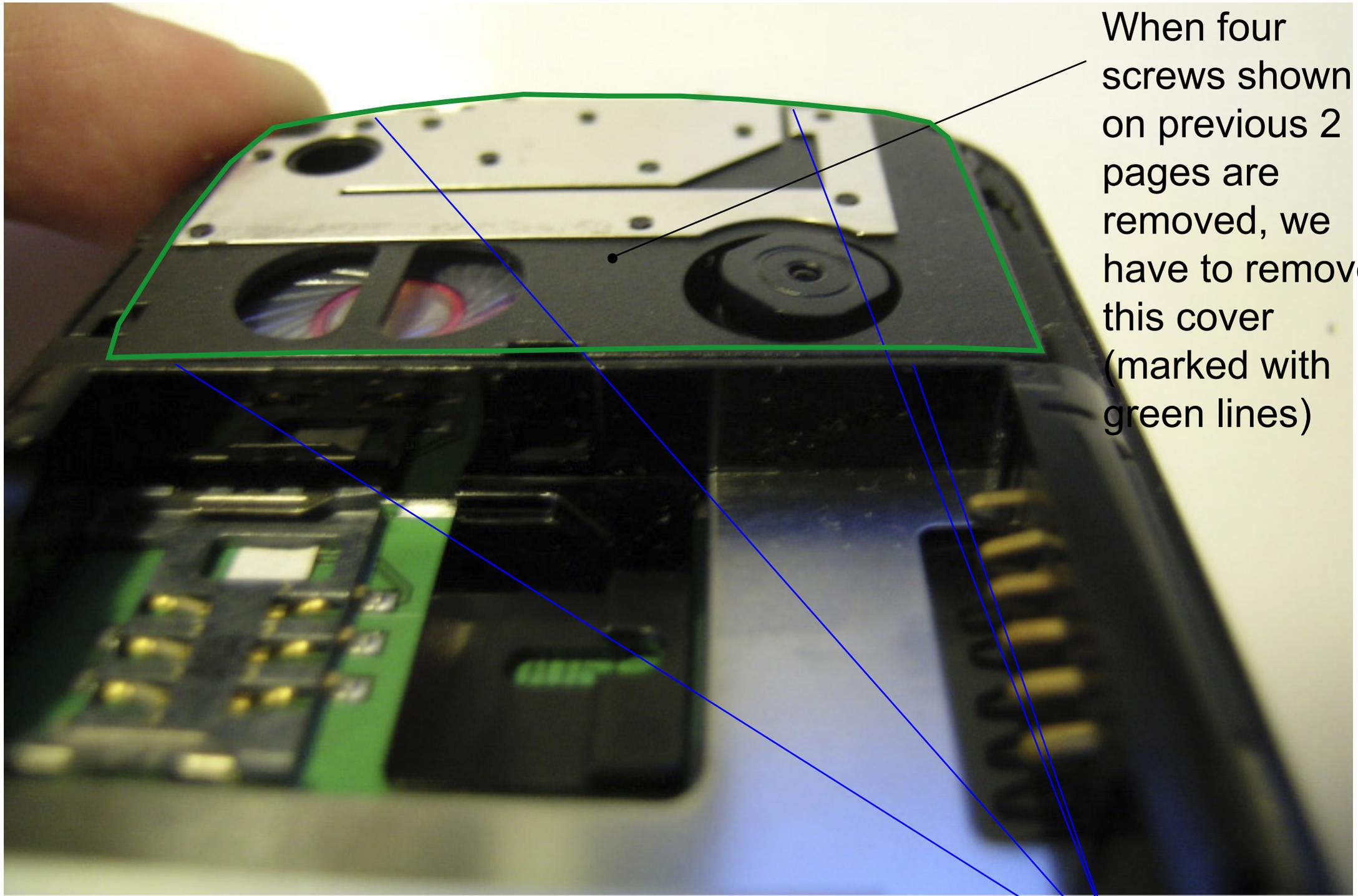
When four screws shown on previous 2 pages are removed, we have to remove this cover (marked with green lines)
