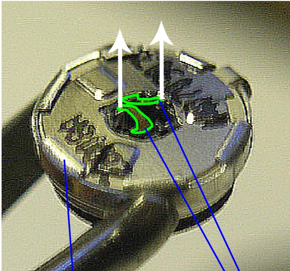
The contacts of the earpiece should be cleaned with ethyl alcohol. Then their raised ends should be raised more in the direction marked with the white arrows.
