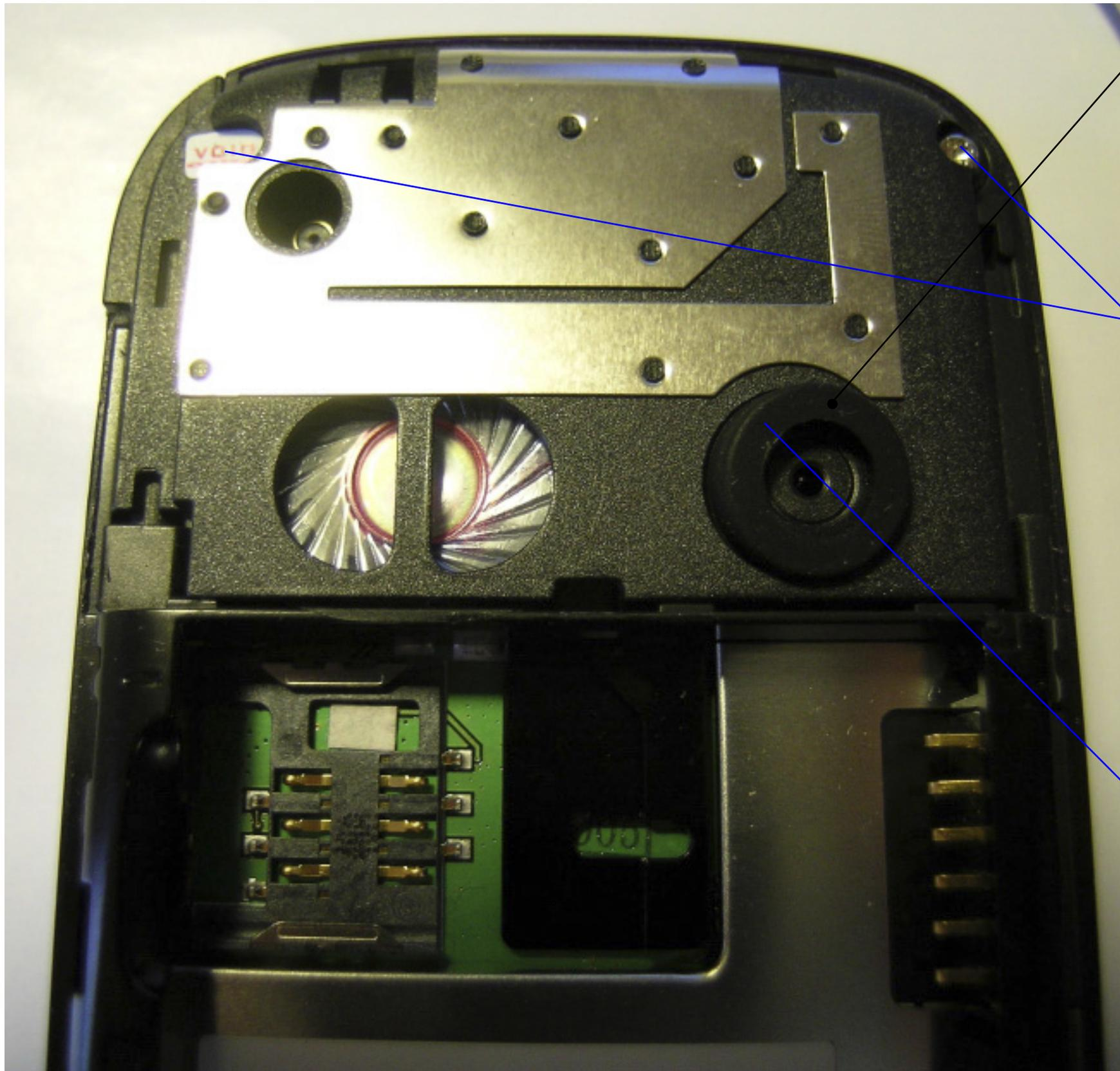
Remove the rubber ring around the camera lens
