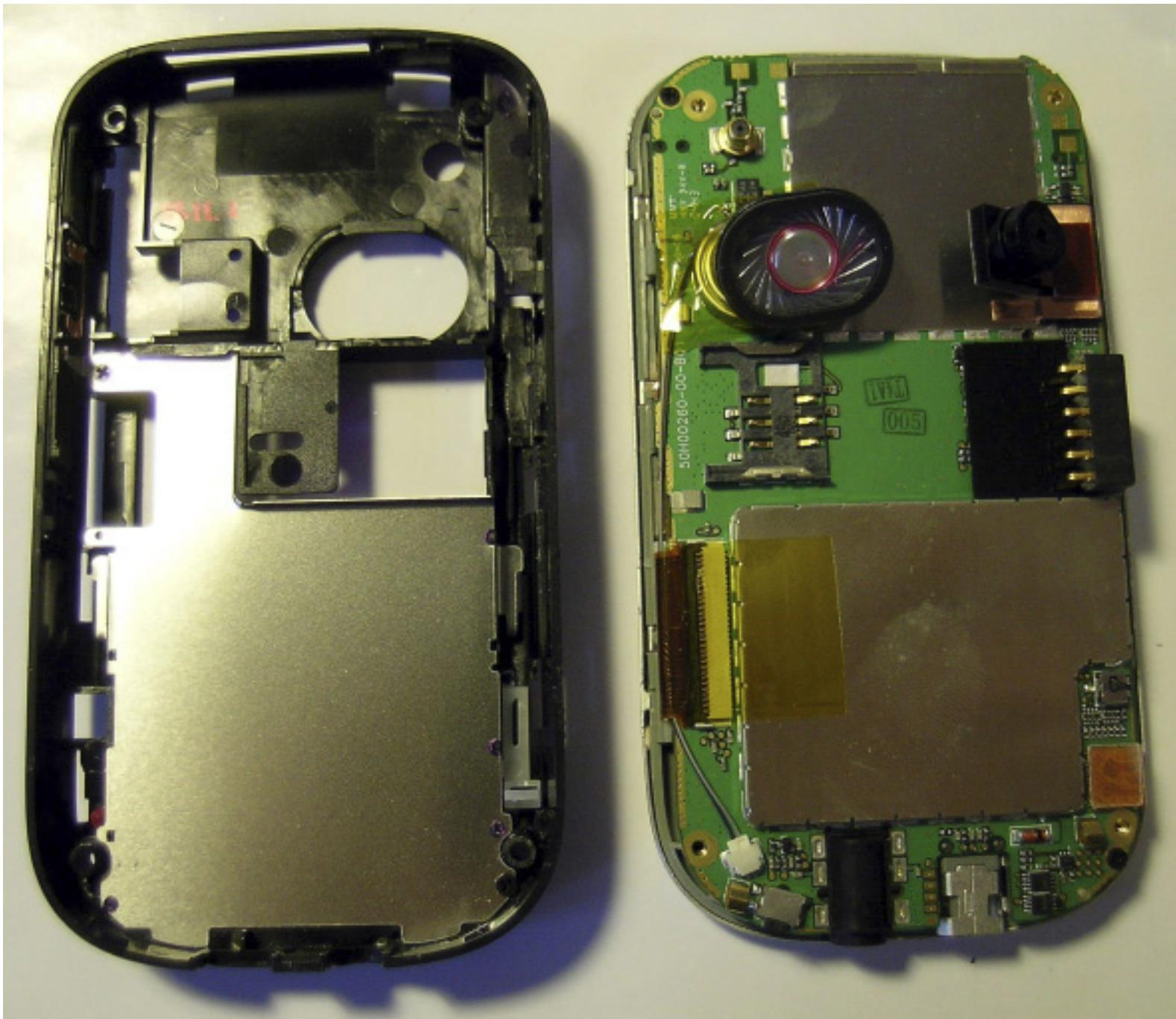
Now we have to remove the side cover which is to the left. The speaker should be raised and put through the opening. The camera can be lifted on the flexible connection in order not to prevent the side cover putting off. The side cover is joined to the base (which is to the right) with hooks on the base. The hooks go to the corresponding
