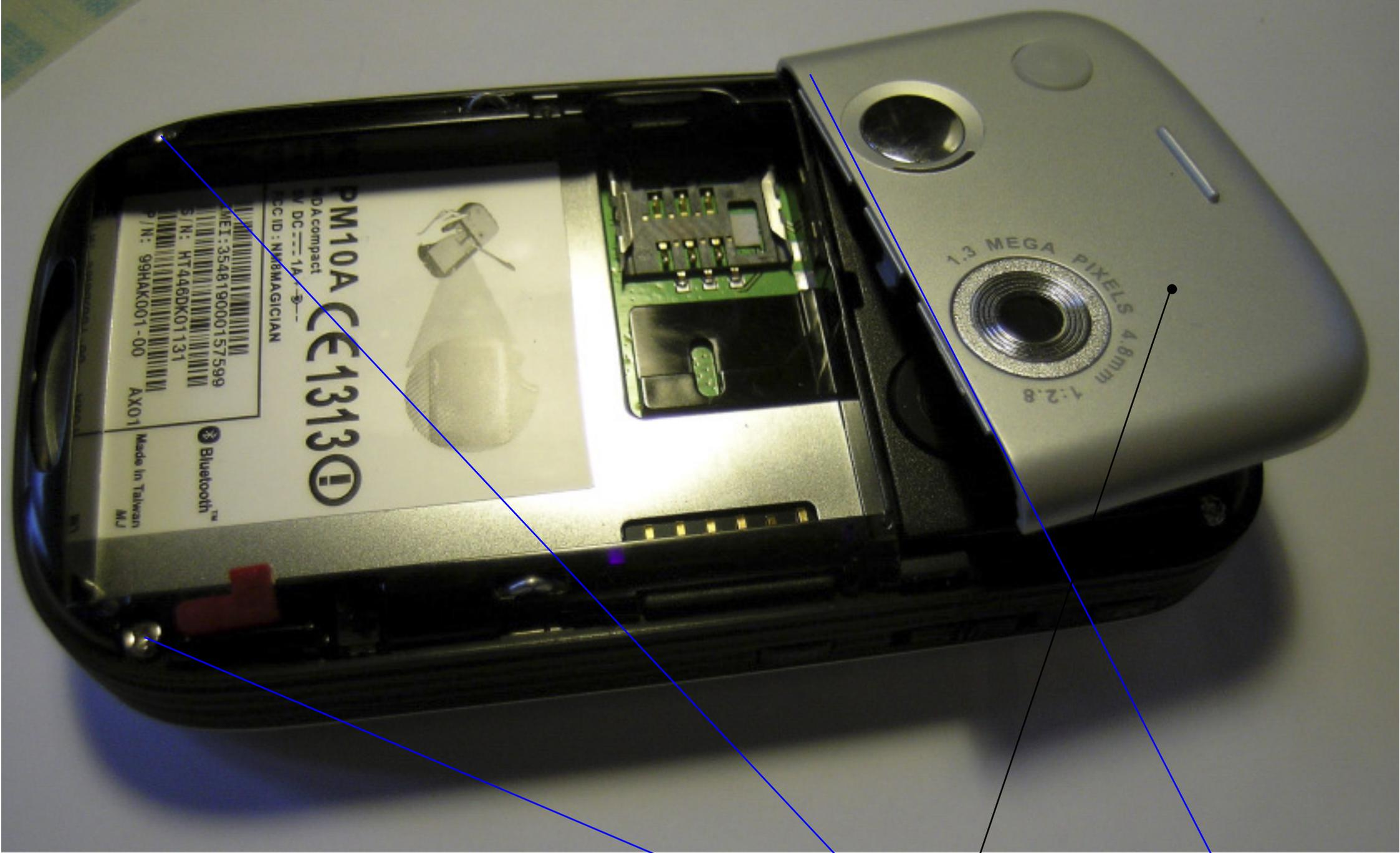
When all but one hook are disconnected the cover will be held by the last one. Slightly rotating the cover and moving to the side disconnect it.
