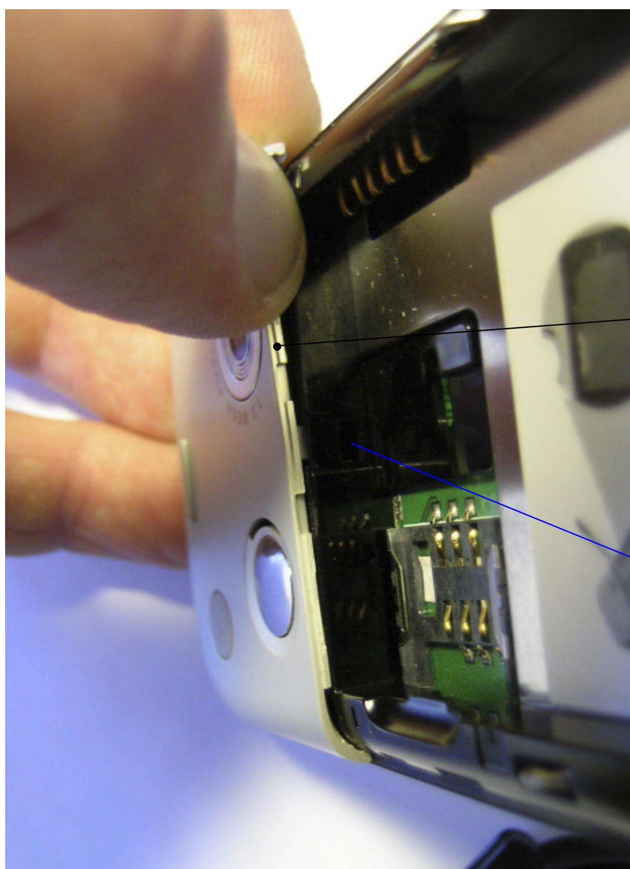
When the cover is raised 3-5 mm from the plastic backside, a hook may become a hindrance. Push it through the opening inside while holding the cover.
