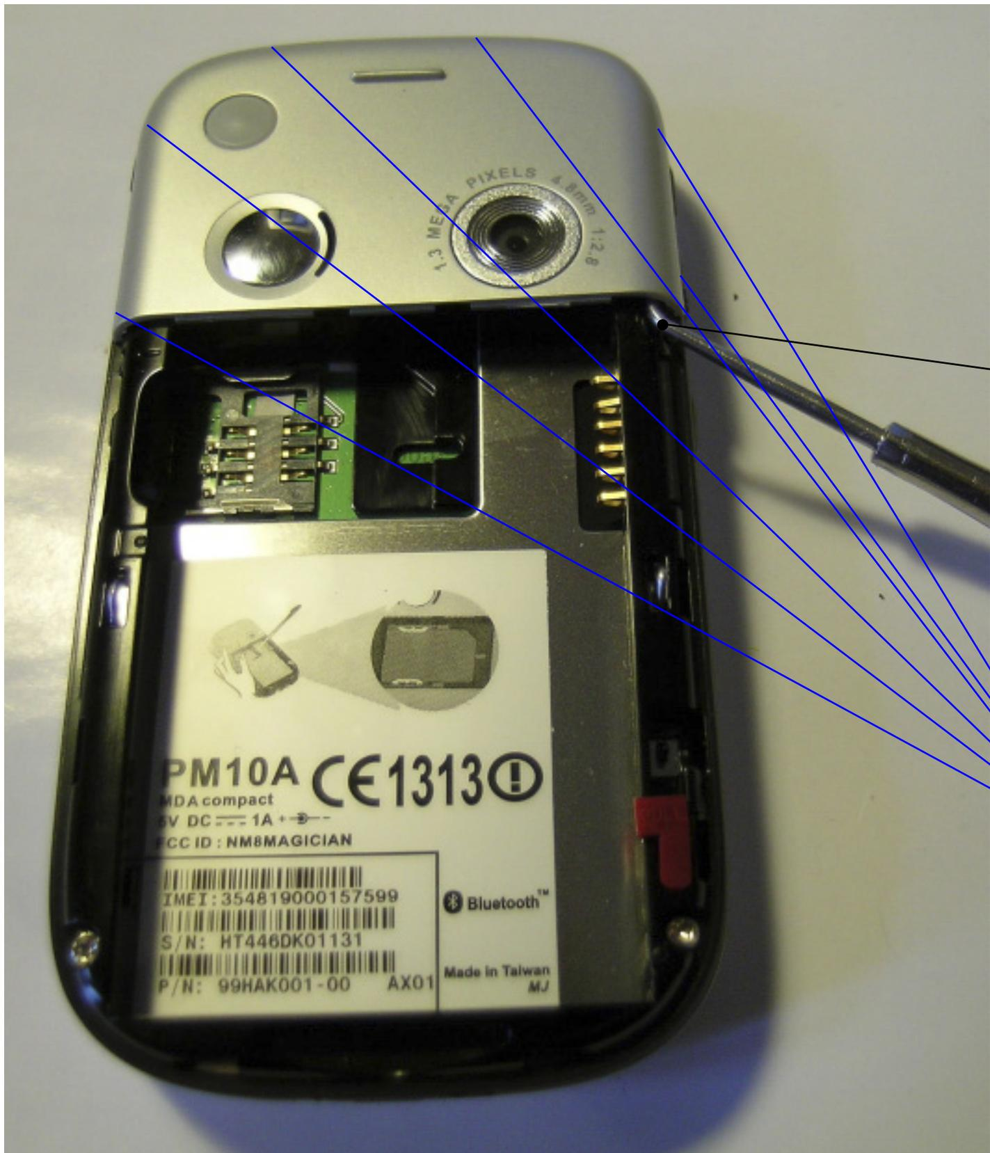
Insert a probing rod here and unhook the cover moving the rod to the right and up. I used a dantist's probe.
